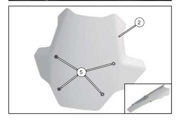
Install the rubber bushings (5) into the corresponding holes on the front windshield (2). CFMOTO
