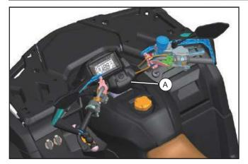
Pull up and remove the handlebar guard (A).
